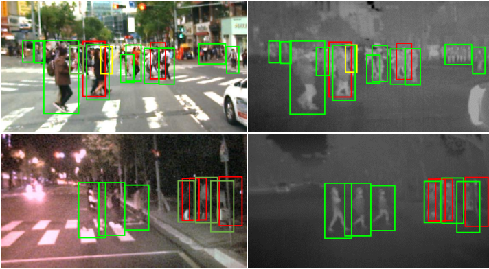
Figure 1: Examples of proposed multispectral pedestrian dataset . It consists of aligned color-thermal image pairs for day and night traffic scenes. The annotations provided with the dataset such as green, yellow, and red boxes indicate no-occlusion, partial occlusion, and heavy occlusion respectively.
